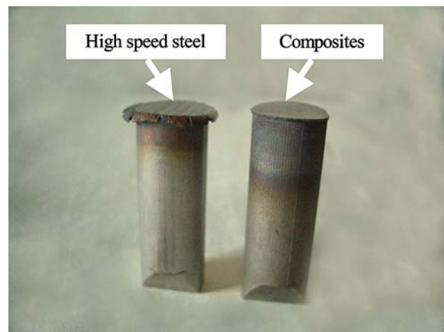
Fig. 4 Wear morphology of the pin samples at 400 °C
